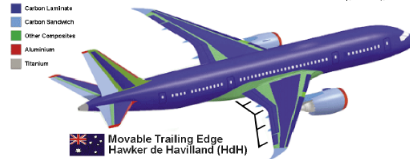
Figure 1: Boeing 787 Dreamliner, showing breakdown of materials used and the MTE designed and manufactured by HdH
