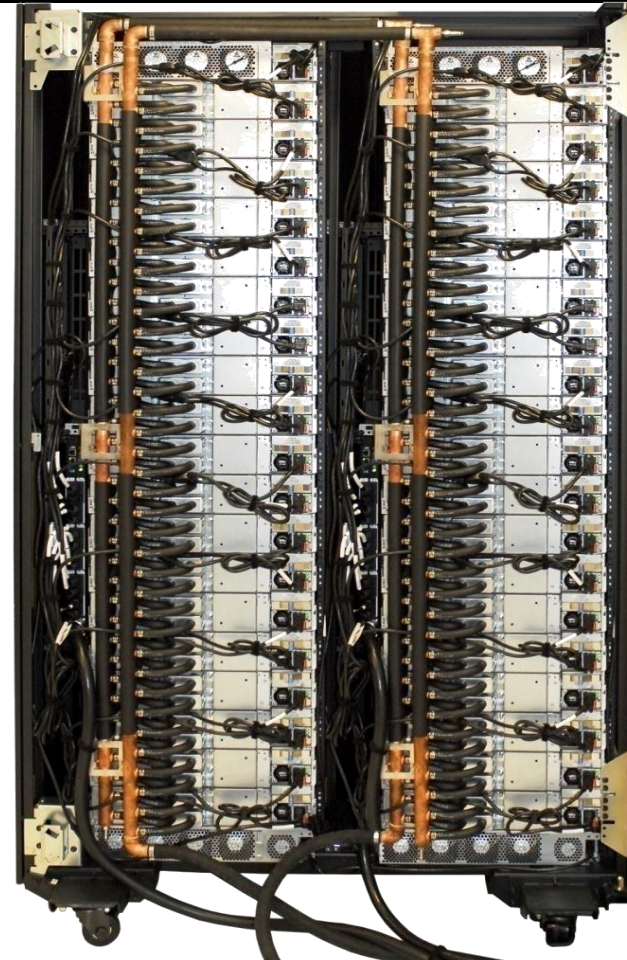
iDataPlex DWC Rack w/ water cooled nodes (rear view of water manifolds)
