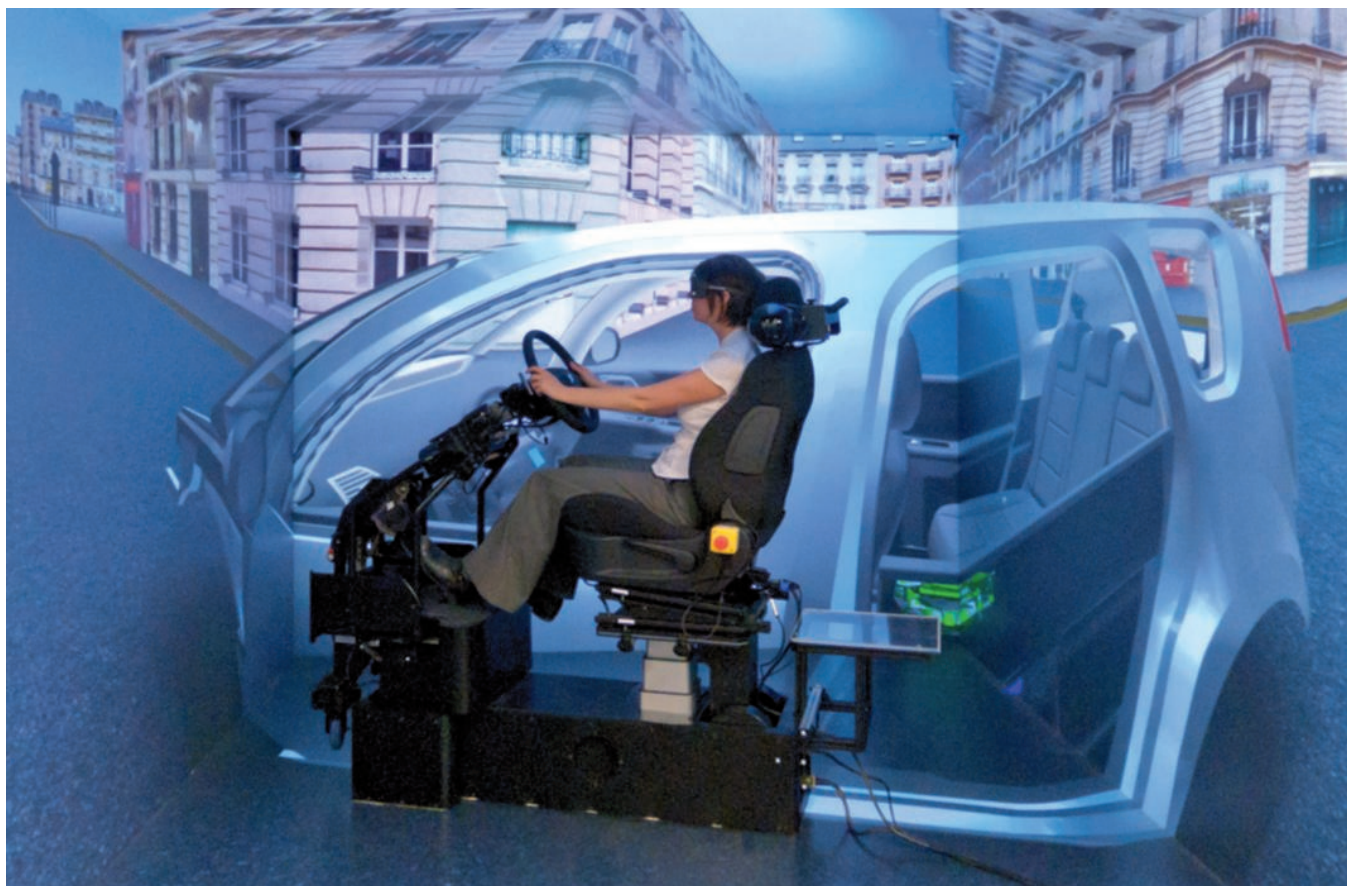
In their CAVE virtual reality room, PSA installed the Holobench, a reduced scale device for working on driving skills in augmented reality (PSA).
