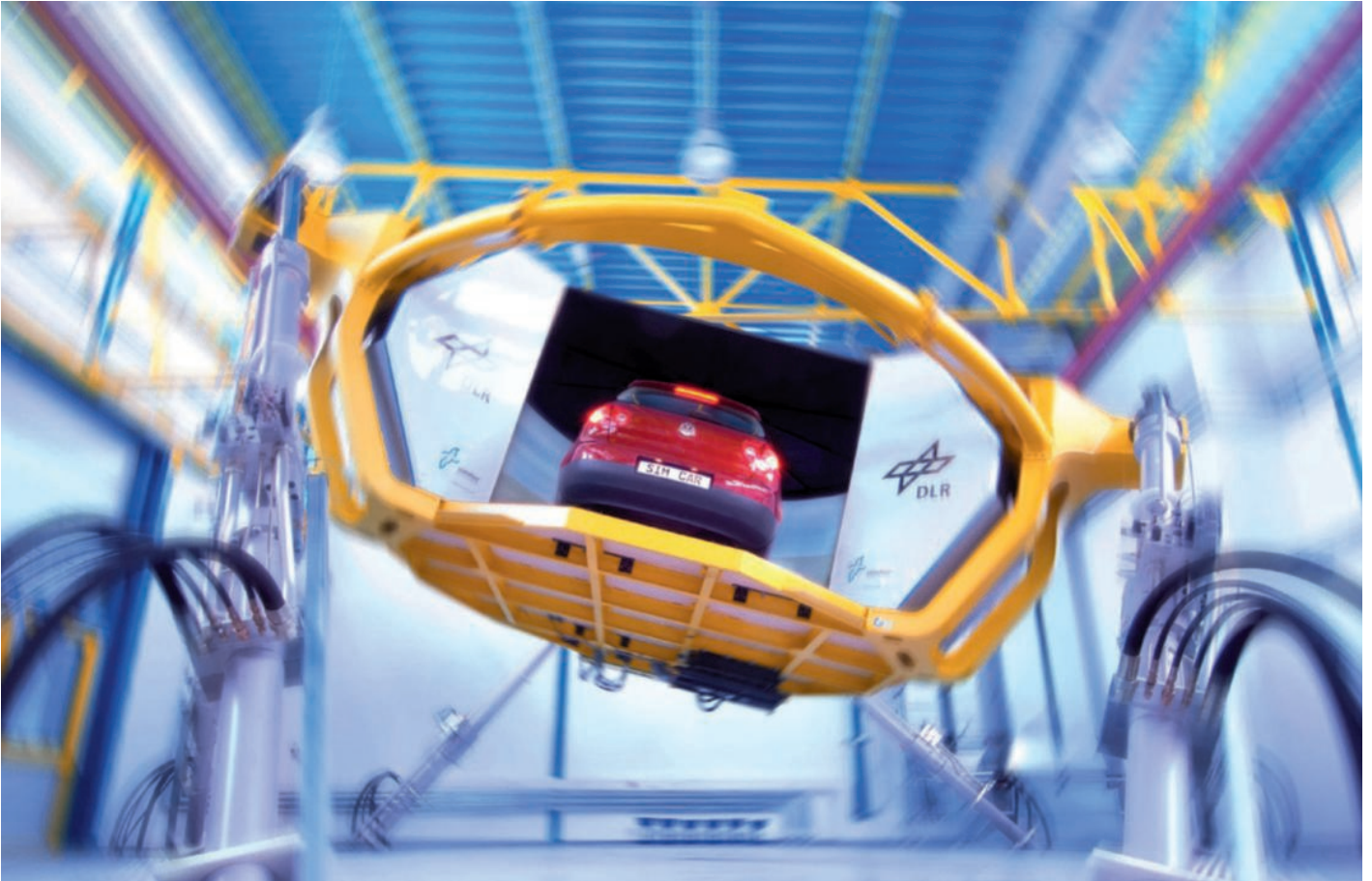
Studying driving on uneven surfaces, thanks to this giant simulator (DLR Institute).
