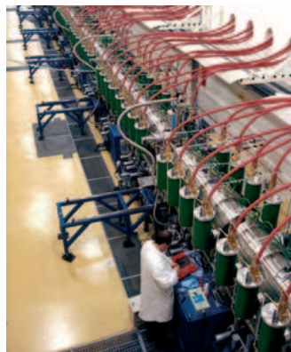
AIRIX the radiograph machine for validating calculations relating to the first step in the functioning of a weapon.
